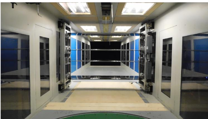
The active multi-blade device installed at the Giovanni Solari Wind Tunnel
