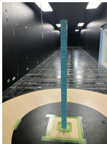
Aeroelastic model of a super tall building in the TPU Wind Tunnel (Japan)
